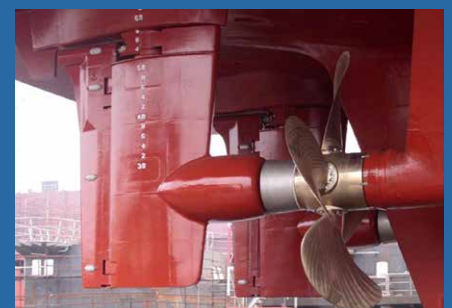
Retrofitted Becker Rudder Bulbs
